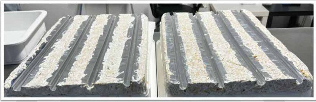
BIOPEX PANEL (BP) = %100 BIOLOGIC (HEMP+MYCELIUM)
